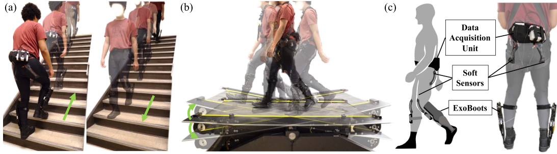
Fig. 3. Experimental setup: (a) Out-of-lab stair trials; (b) in-lab inclined treadmill walking; and (c) soft sensors at hips and knees, along with ExoBoots ankle exoskeletons used solely for ground-truth labeling during stair trials.
